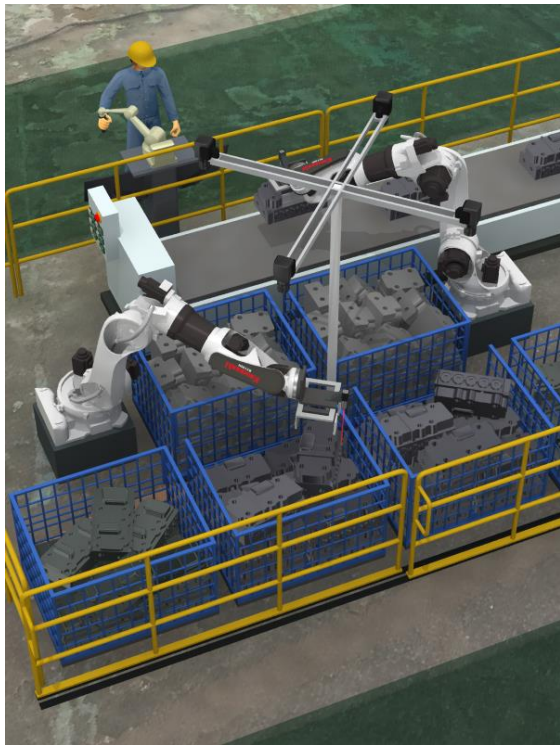
Manual operations only for gripping Automated operations for transfer and loading (Semi-automatic)
