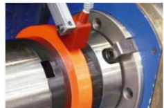
DDU non-contact sensor system with stator and rotor directly on the tool holder
