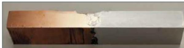
An example of welding between copper and aluminium
