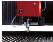
Touch probe Sensor with Anticollision, Laser Painter, and Vacuum Assist
