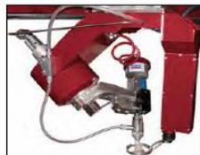
5 axis 3D Evolution  $\pm 69^\circ$  interpolating system with  $\pm 300^\circ$  or infinite (optional) rotation
