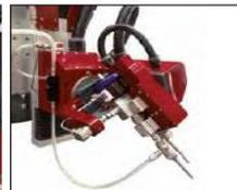
Edge 5 axis  $\pm 55^\circ$  interpolating system with I.T.C.™ (Intelligent Tapering Control)
