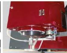
I.T.C.™ - Intelligent Tapering Control system with self positioning touch probe and anticollision device
